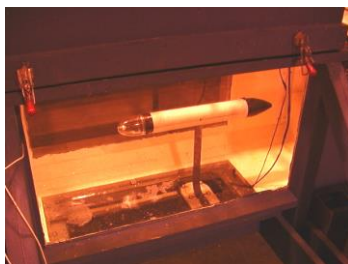
Figure 8: Ranger mockup mounted on six-axis loadcell in flow tank test section
